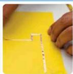
Making a sharp corner: Fold the copper tape back on itself and make a sharp crease. While holding down the crease, turn the tape the direction you would like it to go. Flatten the tape with a bone folder or Popsicle stick.
