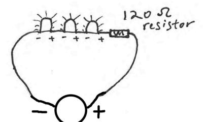
You will be wrapping the wires on the LEDs and solar cell together to make the circuit. Realize that your wraps need to be tight so that the power can flow. Use the wire strippers to peel back the plastic on the wire so that you can wrap it around the legs of the LEDs, resistor and solar cell.
